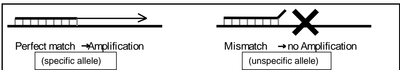
Fig. 1: Principle of SSP-PCR
