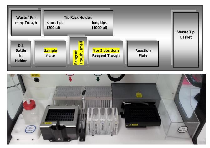
Reagent Position in the 5 positions Reagent Trough for SSO tests:
