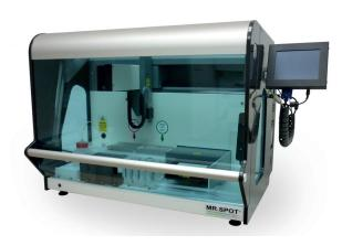
Attach the touch screen using the support arm provided, and connect to the  ${\sf MR.SPOT}^{\circledast}$  Processor with the associated cables.
