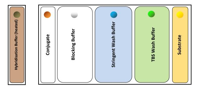
Reagent Position in the 4 positions Reagent Trough for HLA antibody tests:
