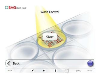
The Wash Program allows cleaning all lines of the MR.SPOT<sup>®</sup> Processor. Press **Start** and follow the instructions on the screen. It is recommended to run a disinfection wash every three months. Disinfectants like Liquinox<sup>®</sup>, Virkon<sup>®</sup>, 1% Chloros<sup>®</sup> or 1% bleach (natriumhypochloride) can be used for the disinfection run.
