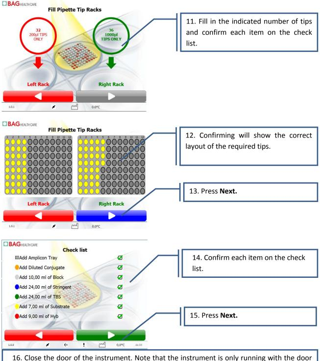
closed. Opening the door during the run will interrupt the assay. It is possible to resume the run after closing the door again.
