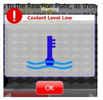
It will appear when you start the MR.SPOT<sup>®</sup> and every time before you try to start a run. If there is not enough coolant the reaction plate will not be cooled fast enough, resulting in false negative reactions. Please fill up the coolant or contact your local representative to do so!
